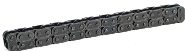
CATENA 7MM / 22 INNESTI / 44 MAGLIE 7 MM CHAIN / 22 SPROCKET TEETH / 44 LINKS
